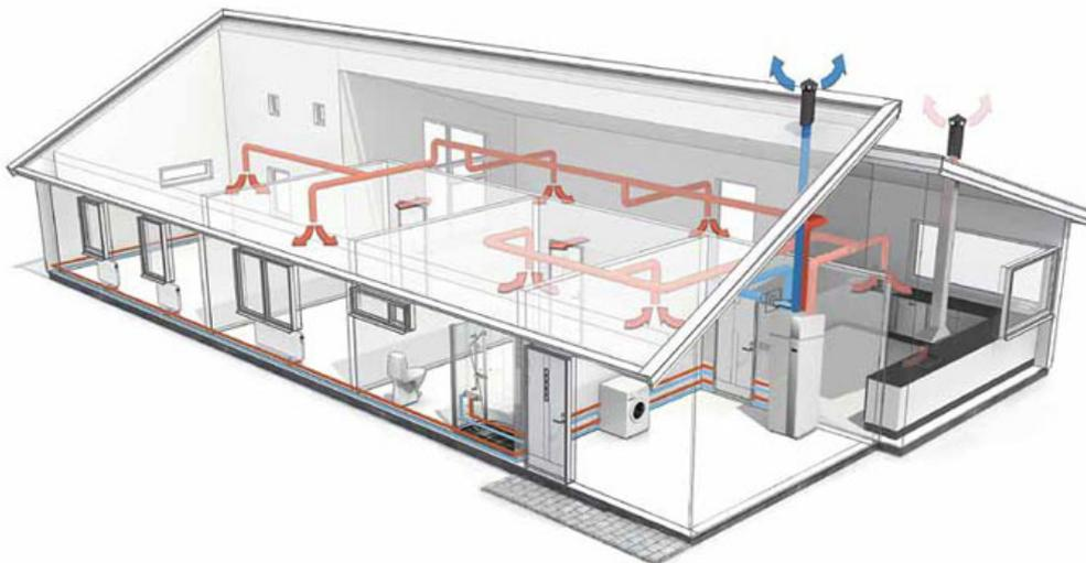
Figure 1: Typical Exhaust Air Source HP arrangement
