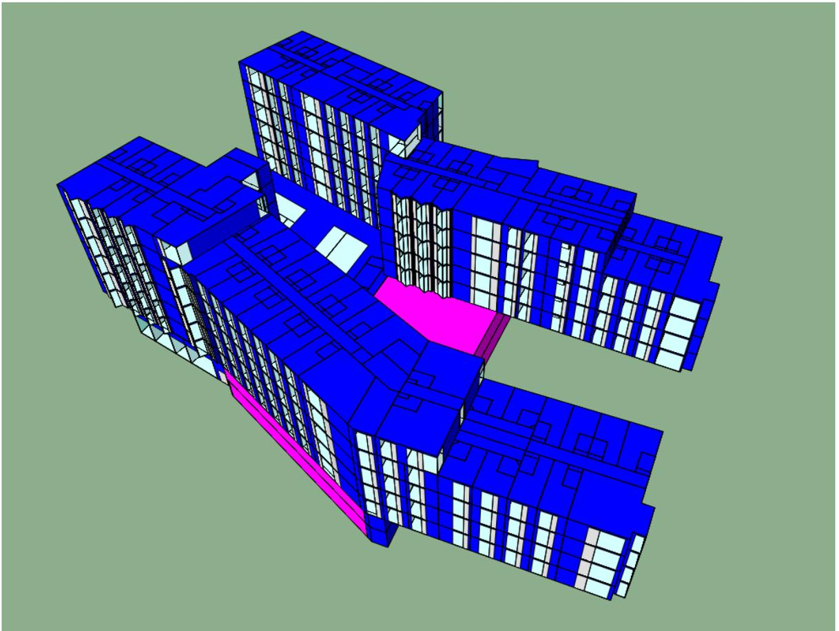
**Figure 4.0.1** – 3D model image for the IES VE Building Performance Simulation model for the Phibsborough Shared Living Development. The software is approved by the SEAI for Part L and BER calculations.
