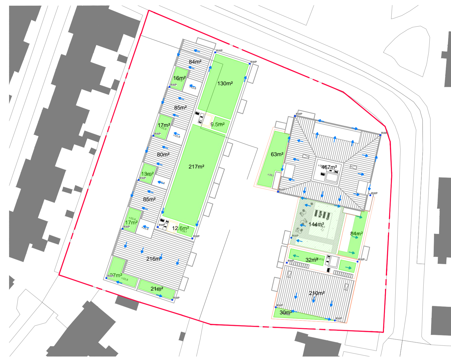
ROOF LEVEL FLOW PATHS SCALE 1:500
