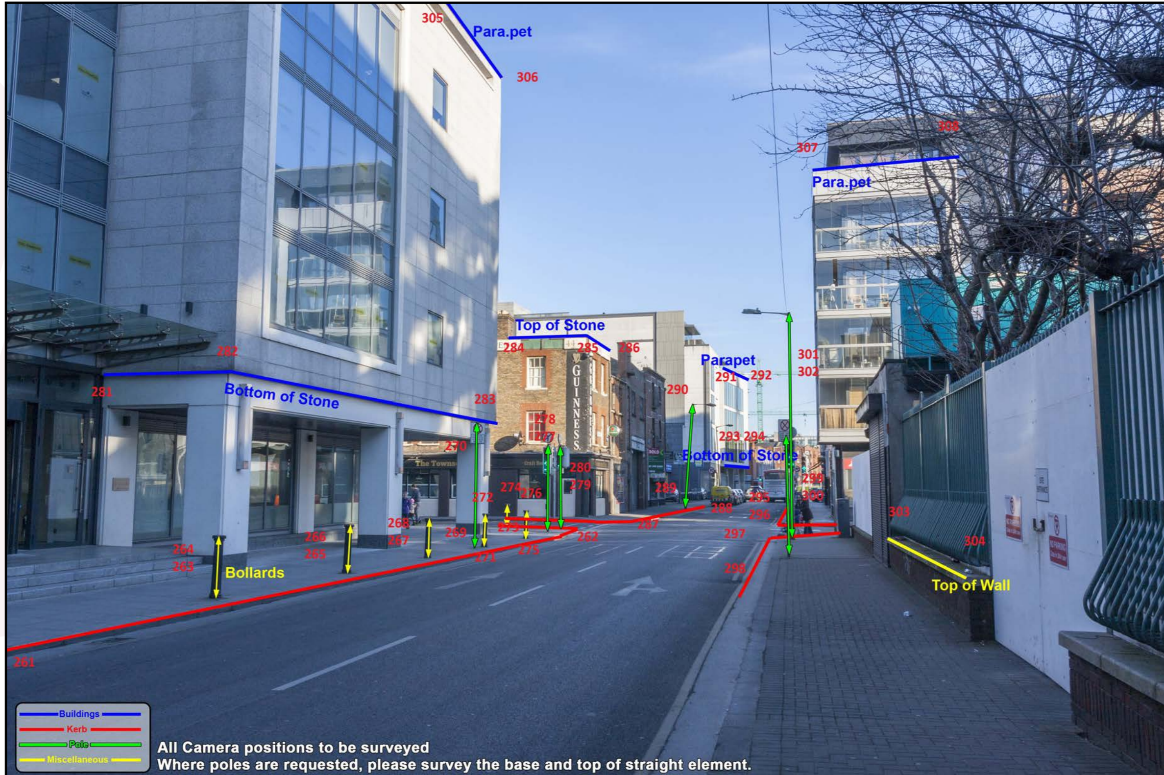
Fig.10: Fixed reference points for surveyor on Baseline untreated photo.
